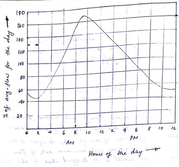
The hourly, daily & seasonal variations of sewage flow (OWF) of a town affects the working of not only sewers but also the pumping stations and treatment plant. The hourly rate of waste water flow is affected by the hourly variations in water consumption. In general the waste water discharge curve closely follows the water consumption curve but with a time lag of few hrs.
